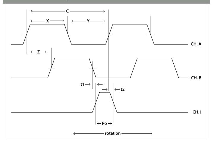
A leads B for clockwise shaft rotation, B leads A for counter clockwise shaft rotation viewed from the cover side of the encoder.
